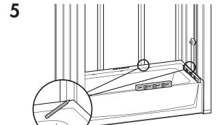
Level and mark all sides. Front apron should be firmly on the floor.
