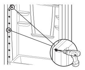
Fasten flanges along top of left side wall with fasteners of choice (see Pre-Installation Planning #12) into each corresponding stud. Fasten side (vertical) flanges to side studs 8" (200mm) on center. NOTE: Finish caulking is not required, however, if using caulk, weep channel must remain clear of obstruction to allow for proper drainage of the unit.
