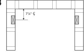
Additional stud may be required for vertical backwall flange. Stud @ 7% CL from back, on both sides. Stud can be turned for easier installation.
