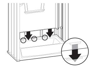
Lift and place back wall, making sure locking tab is engaged.
