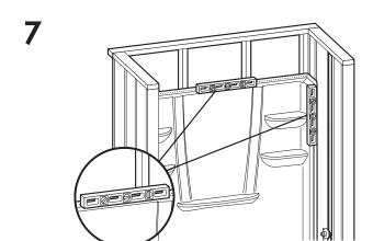
Level back wall vertically & horizontally. Shim if necessary.
