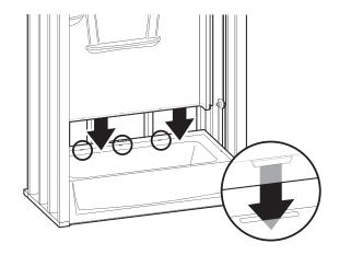
Lift and place the back wall, making sure locking tabs are engaged.
