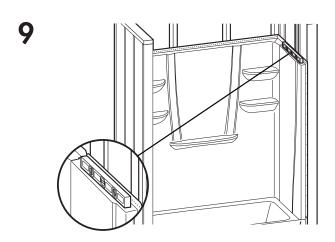
Check for level. Shim if necessary.
