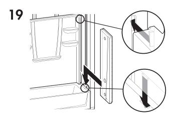
Slide right side wall into position. Be sure locking mechanism is engaged. **NOTE:** Finish caulking is not required, however, if using caulk, weep channel must remain clear of obstruction to allow for proper drainage of the unit.
