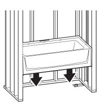
Install drain assembly per manufacturer's instructions. Place base into framing pocket.
