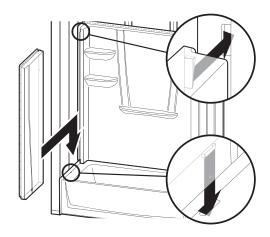
Slide left side wall into position. Be sure locking mechanism is engaged. NOTE: To accommodate any stud variation, you may have to add a bead of waterproof adhesive such as 100% silicone to eliminate any potential free play. 23
