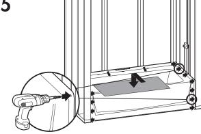
Pre-drill horizontal flanges along top of base section and fasten into each corresponding stud. Pre-drill both (vertical) side flanges and fasten to side studs 8" (200mm) on center. Place cardboard to protect finish.
