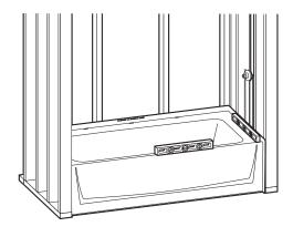
Level lengthwise and widthwise using 3 ft. (915mm) level by shimming if necessary. The unit must be set level.
