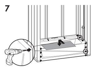
Pre-drill horizontal flanges along top of base section and fasten into each corresponding stud. Pre-drill both (vertical) side flanges and fasten to side studs 8" (200mm) on center. Place cardboard to protect finish.
