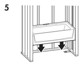
Install drain assembly per manufacturer's instructions. Place base into framing pocket.
